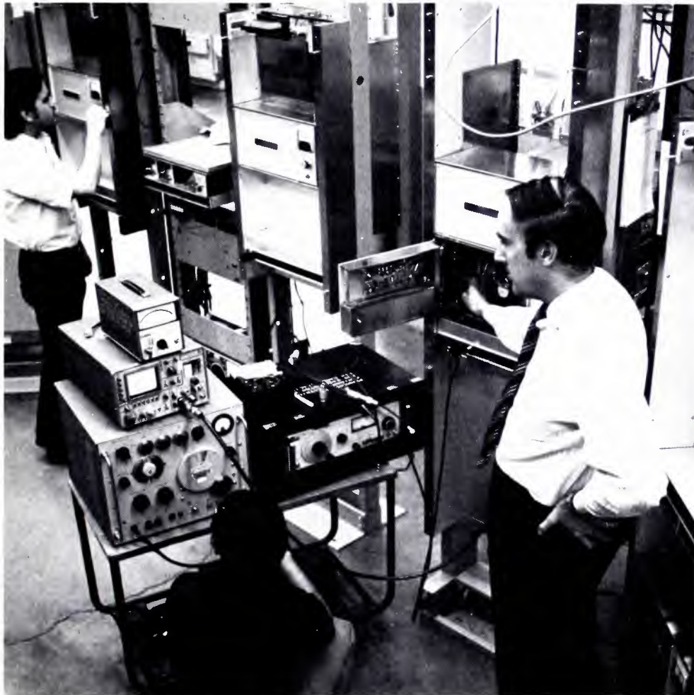
The equipment shown here in system test is part of a microwave network which extends CPB programming from Sprague, Washington to ETV stations in Pullman, Washington and Moscow, Idaho.
